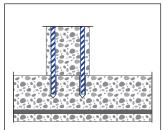
Overlap joints for slabs and beams or foundation column or wall; rebar connection for simply supported slabs or beams; shear connector or compression component joints.
