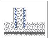
Overlap joints for slabs and beams or foundation column or wall; rebar connection for simply supported slabs or beams; shear connector or compression component joints. Important note: Architect or design engineer must conduct final checked with the actual site condition for any variations against tabulated data.
